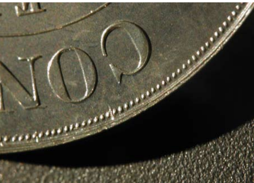
Above: Die Gouge on Bashlow restrikes. Photos: Jeff Shevlin.
